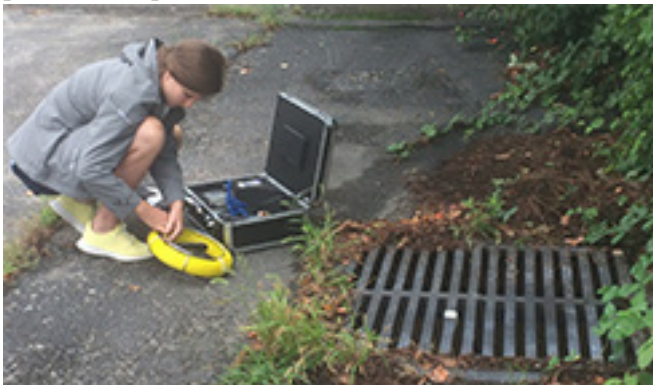
UT student and Farragut resident, Caroline Stephens, prepares a snake camera to inspect the inside of this catch basin.
