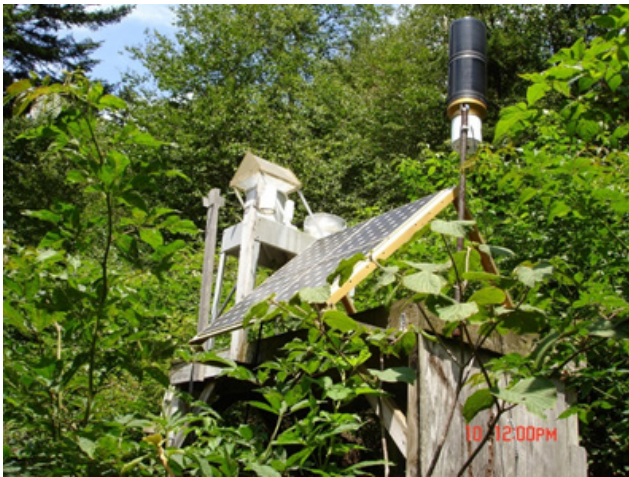
Open site deposition collector and full weather station at the high-elevation Noland Divide Watershed Research Site. Note: vegetation has been cleared since photo was taken for routine site maintenance.
