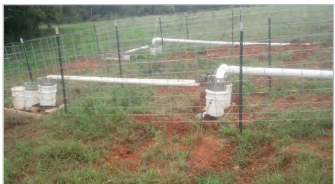
Pinson et al. (2003) flow divider buckets monitoring sediment from cow paths.
