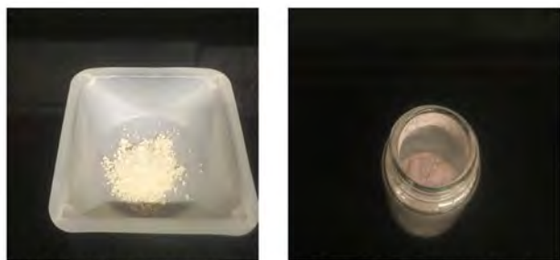
Figure 2 — Diatom powder used in this study is shown. The color change from off-white to light purple indicates the crown ether attachment
