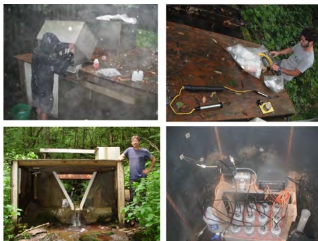
Figure 2. Photos of the Noland Divide Watershed, high-elevation monitoring station in the Great Smoky Mountains National Park. From upper left to lower right, MS student Andrew Veeneman calibrating a water quality sonde at a H-flume, and installing a new pressure transducer at the same site; Dr. John Schwartz at one of the two 3-ft H-flumes, and the instrumentation in the soil lysimeter pit.
