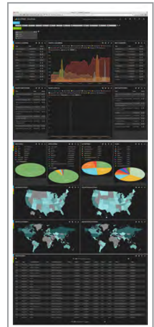
GLORIAD InSight System. A sample analytic dashboard illustrating near-real-time updates of live traffic flows and including country-level summarization, average packet loss, protocol, application and various performance flags, source/destination by US state and country and individual flow records.
